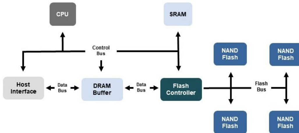
Figure 1: Simple SSD Block Diagram. The diagram above shows the main components of an SSD, which consists of the host interface, the controller, a data buffer, optional SRAM/DRAM, and the flash array.
