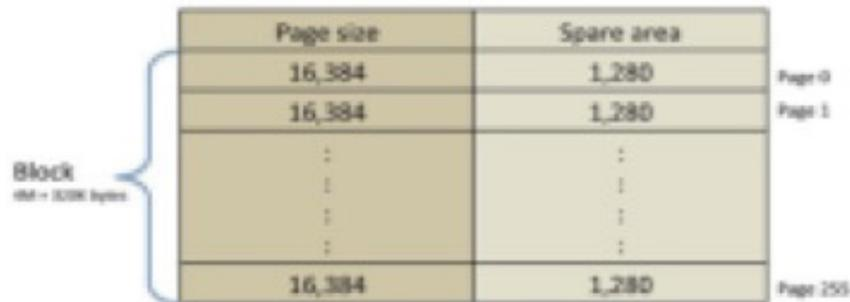
Figure 2: Block and Page Structure of a 16K Page NAND Flash Drivemponents of an SSD.
