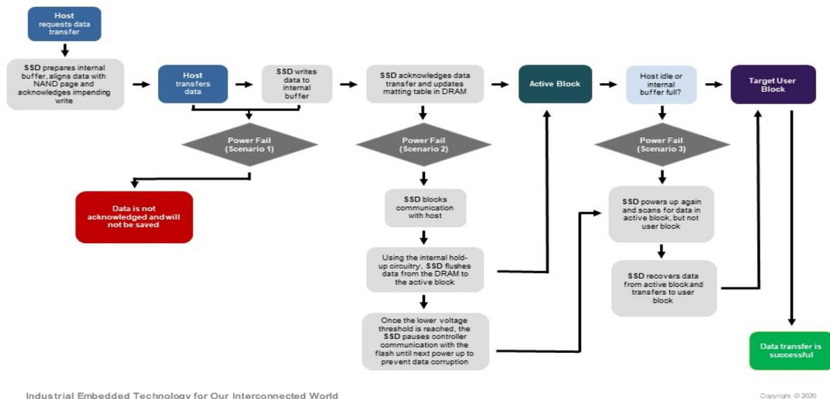
Figure 3: Power Failure Scenarios and vtGuard Protection Mechanisms
