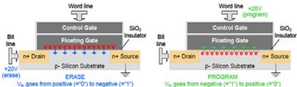
Figure 1: The Floating-gate Transistor
