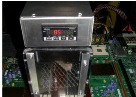
Testing Memory Modules at + 85°C
