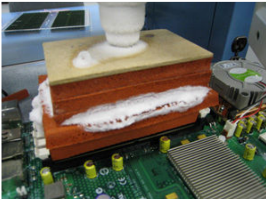
Testing Memory Modules at - 40°C
